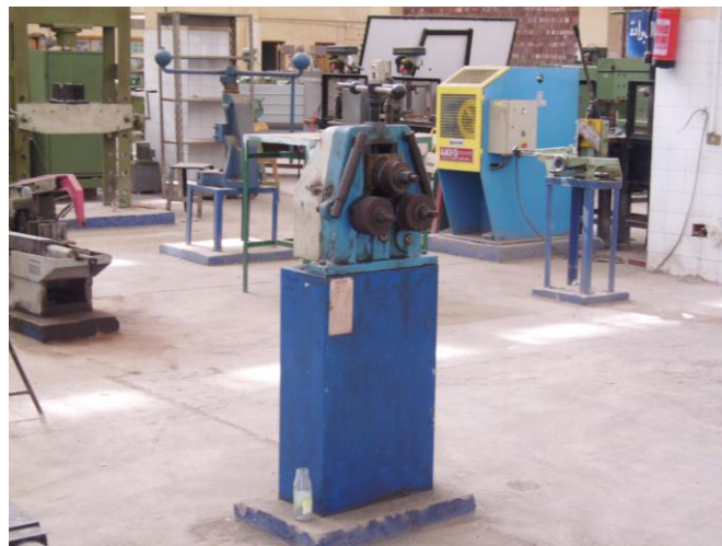
Fig. 2 Section and Pipe Bending Machine
